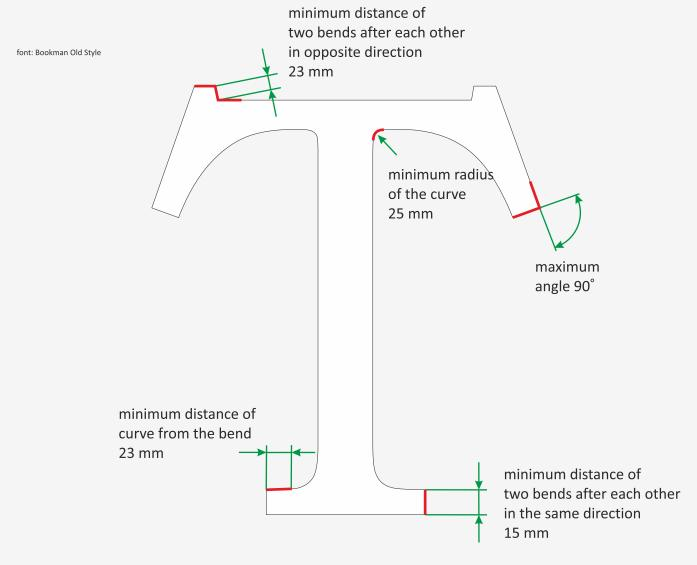
**NOTE**: Machine settings allows making of preliminary bends and increase minimum values of distance of bends from bends and bends from curves.
